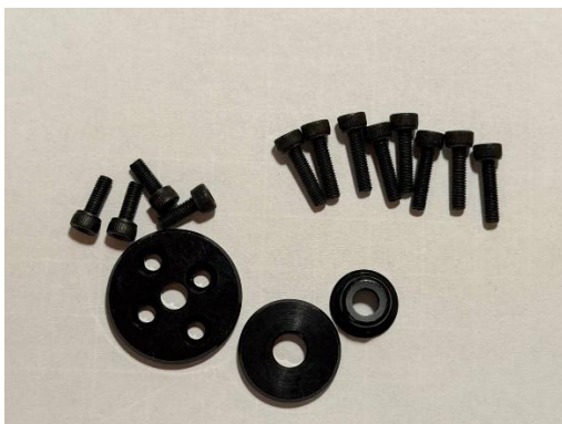
Fig. 12. Propellers mount set (M3 x 8 mm 4 pcs, M3 x 12mm 8 pcs)
