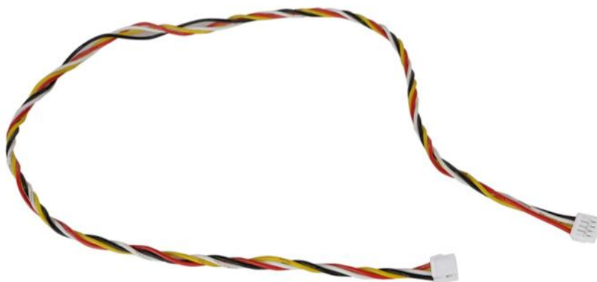
Мал.1. Pitot cable JST-GH 1.25 4pin JST-GH 1.25 4pin 30AWG 400mm
