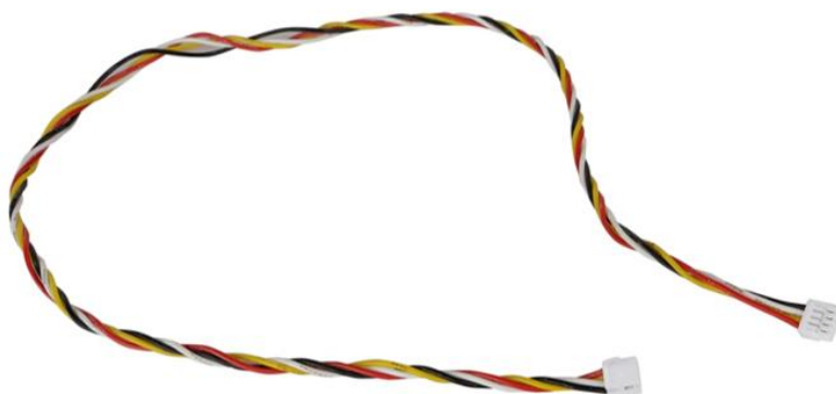
Fig.1. Pitot cable JST-GH 1.25 4pin JST-GH 1.25 4pin 30AWG 400mm
