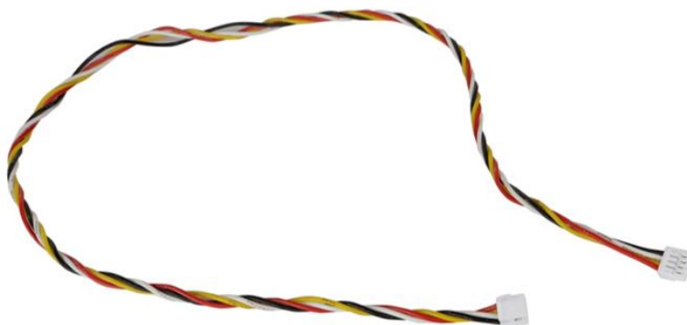
Abb.1. Pitot cable JST-GH 1.25 4pin JST-GH 1.25 4pin 30AWG 400mm
